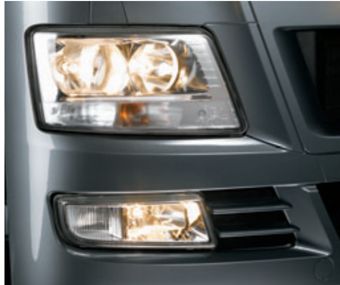
Headlights with free-form reflectors, Xenon dipped light.
