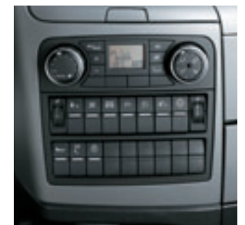
New controls for the air conditioner, heater and ventilation. New switch field with function displays.
