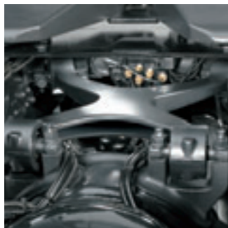
Weight-saving X control arm on the rear axle takes over the stabiliser and control arm functions.
