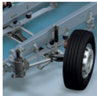
New single-leaf suspension with direct steering for 4x2 semitrailer tractors.
