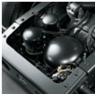
Compressed air tanks situated at the rear.
