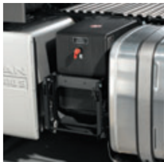
Compact battery box.
