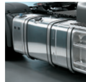
Combination tank for diesel and AdBlue®.
